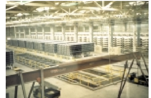
The world's largest reverse osmosis plant in Yuma, USA, is used to reduce the salinity of the Colorado River 270,000 m 3 /d (72mgd)
